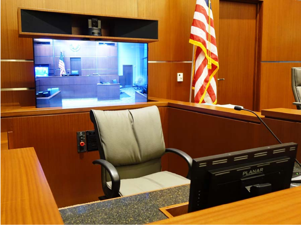
Casework Design that Integrates a Pop-up Display and camera for use with Witnesses Appearing Remotely
