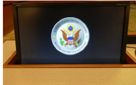
Partially recessed Display improves sightlines over its top
