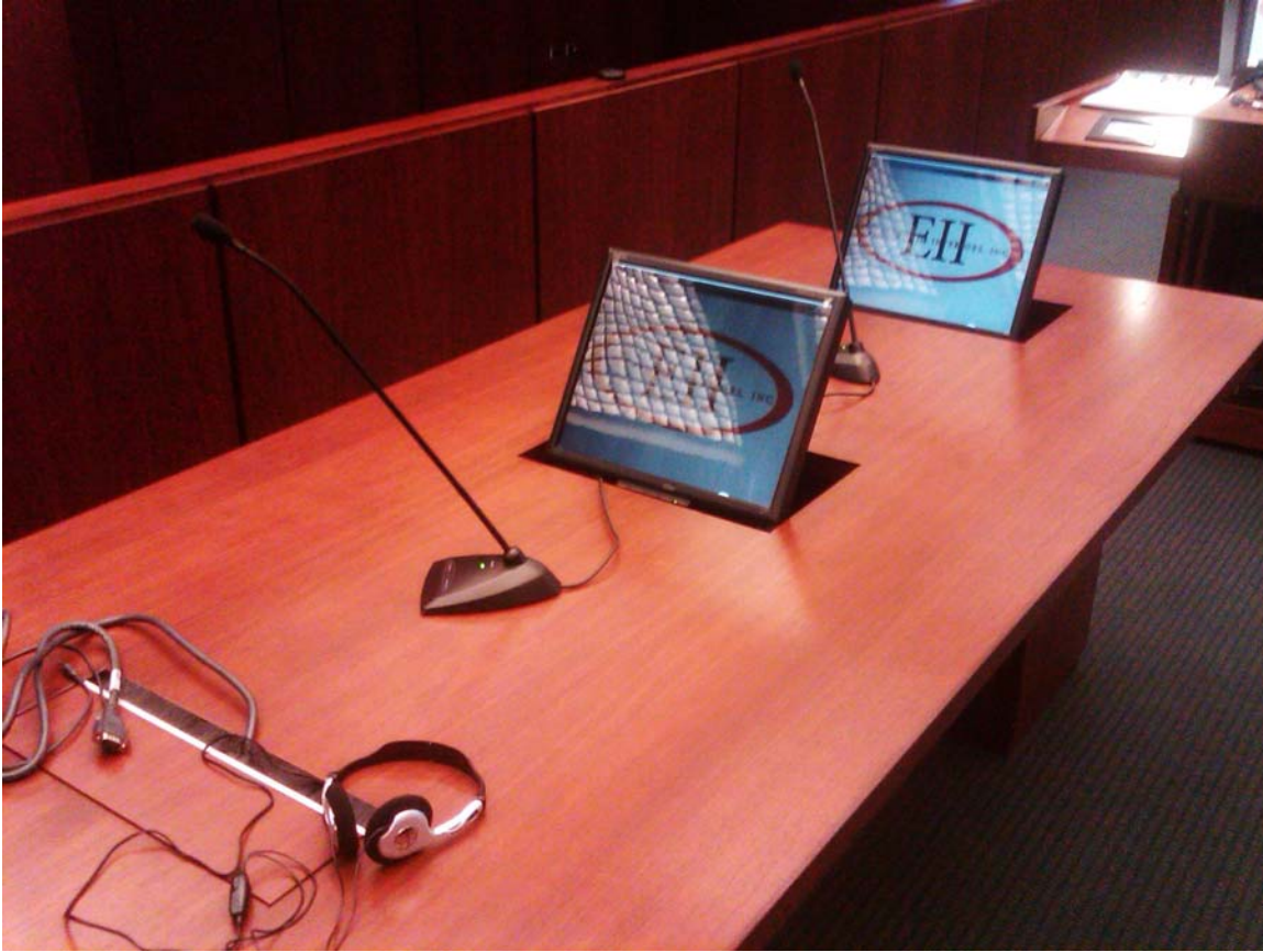
Custom Designed Ambidextrous Smart Table. Note Recessed Displays, video presentation and Headphone Connections
